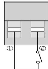
Normally, pin1 and pin2 are connected so that the machine can be working normally. When some emergencies happen, and when users have to cut off the output, just need to disconnect the connection between pin1 and pin2, or just pulling it out.
